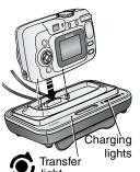
3 Match the connector and alignment pins on the camera dock to the camera. Push down until the camera is securely seated.
